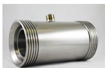
Made from high strength A-286 alloy steel, the meter body is rated to a full 15,000 PSIG for conventional service and 10,000 PSIG for sour service. The new size is an extension to the very successful Hoffer Wing Nut Meter Series (1" to 3" sizes) used extensively in oil and gas well servicing and reflects Hoffer's commitment to meeting new customer needs.
